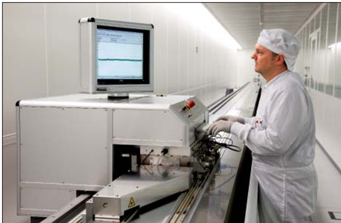
30 m long measuring machine for scale tapes
