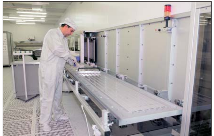
Vacuum machine for application of chromium layers
